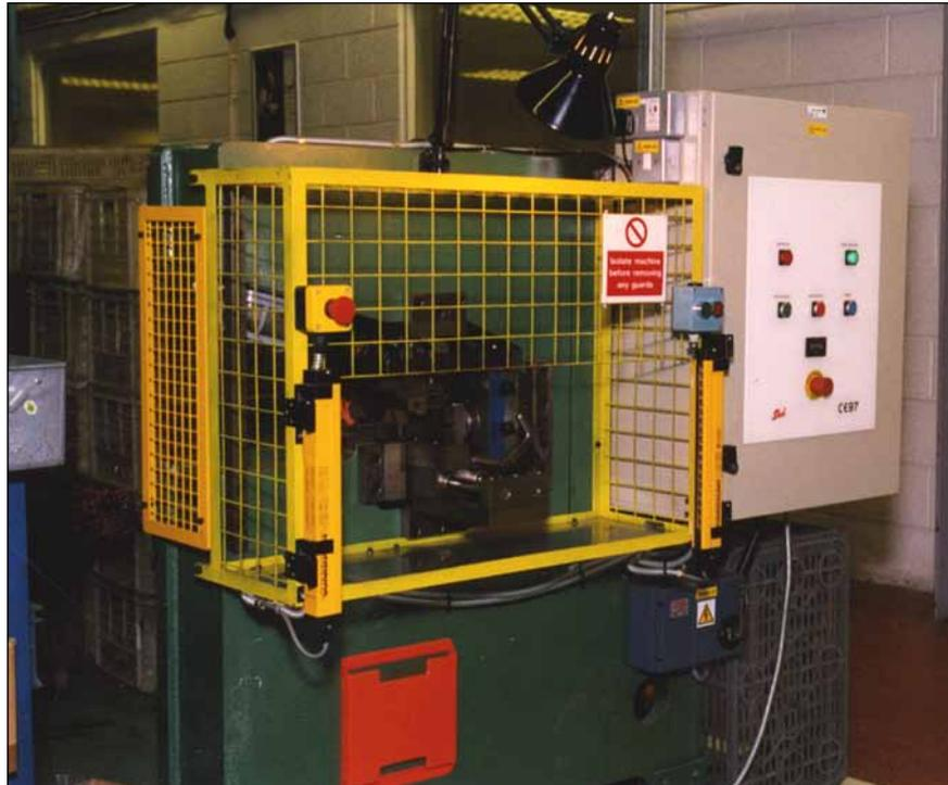
Test rig with combination of protective measures including light curtain
