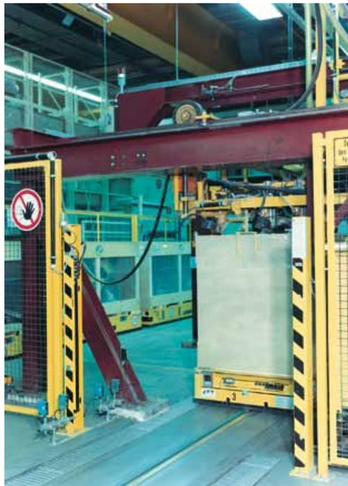
**Entry-exit system. Four beam muting, three beam guard**
