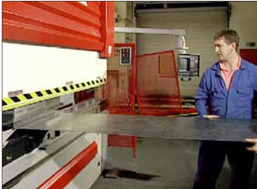
Hydraulic press brake with horizontal light curtain
