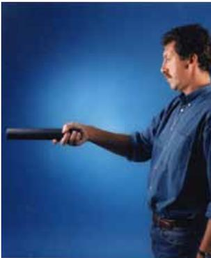
Insert the appropriate diameter test piece into the light curtain
