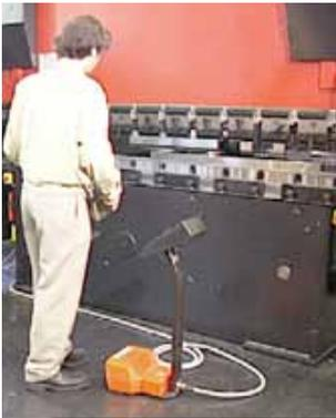
Combined vertical and horizontal light curtain applied to a hydraulic press brake
