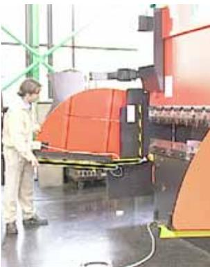
Light curtain which can have its assembly rotated to alter the angle of approach
