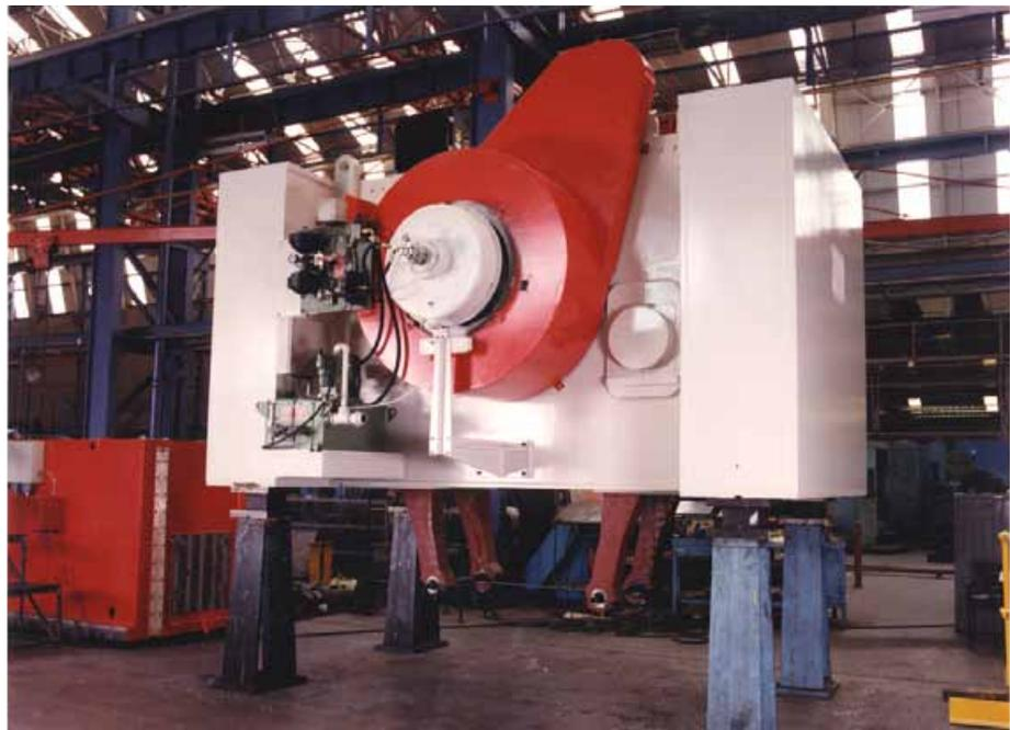
Clutch-brake unit for large power press
