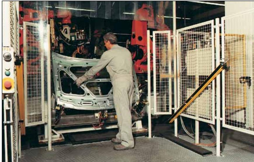
**Robot load bay with Type 4 ESPE**
