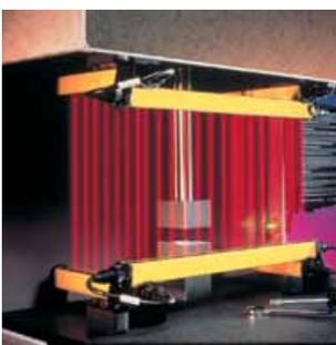
**Minimum separation distance must be calculated to allow safe application of the light curtain**
