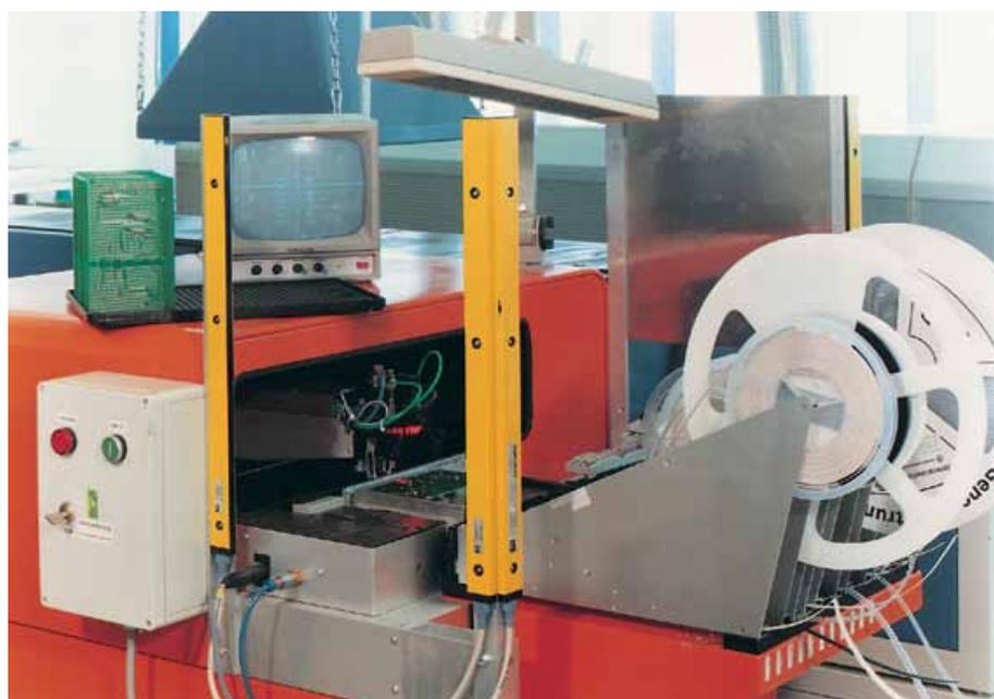
**Three corner Type 2 testing fixture. Additional screens and guards may be required for safe operation in some AOPD applications**
