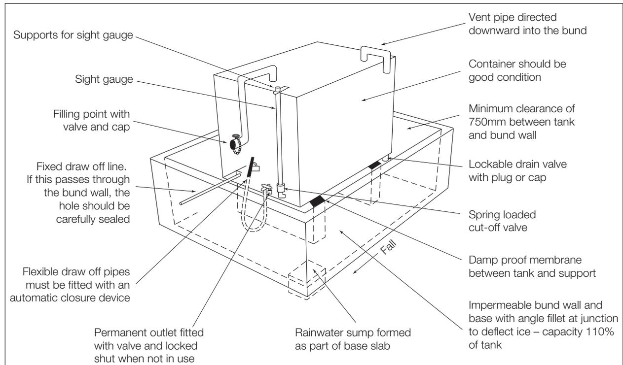
**Figure 1: Banded oil tank (from Environment Agency publication Above Ground Oil Storage Tanks, PPG2 (ref 21))**
